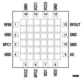
Figure 2. SKY65370-11 Pinout – 16-Pin MCM (Top View)
